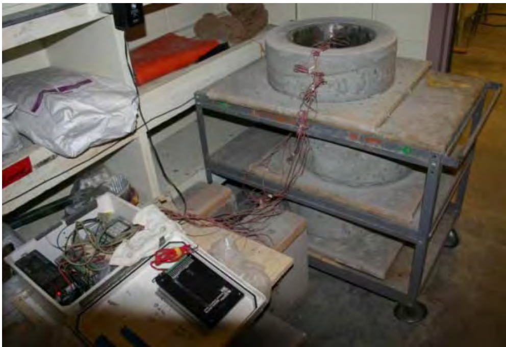
Figure 7.39 Photograph of Restrained Ring Shrinkage Specimen (ASTM C 1581, AASHTO PP34)
